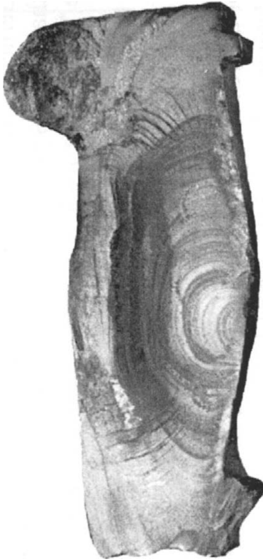
Figure 29.13 Fatigue fracture surface from the broken tyre.
