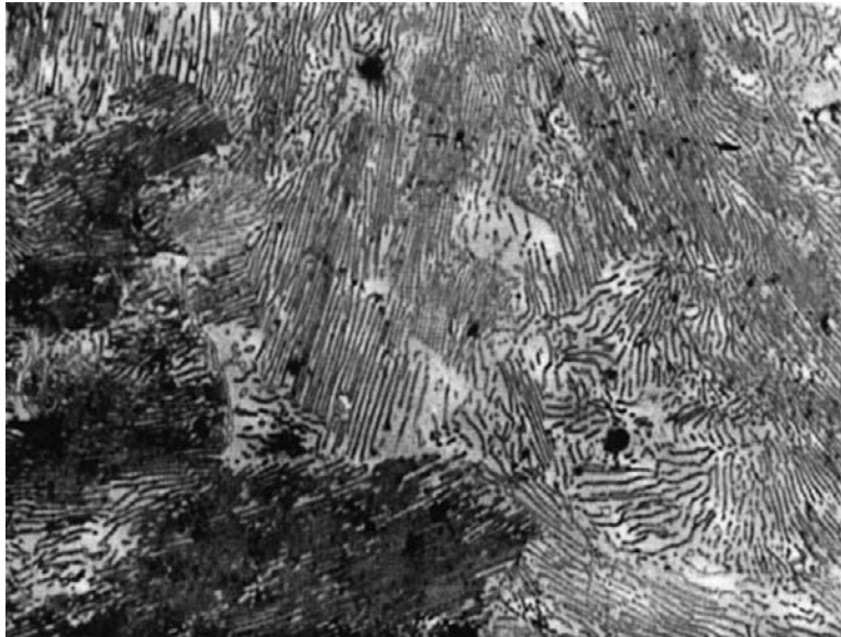
Figure A1.41 Pearlite in a eutectoid-composition plain-carbon steel, \times 500 . (After K. J. Pascoe, An Introduction to the Properties of Engineering Materials , Van Nostrand Reinhold, London, 1978.)
